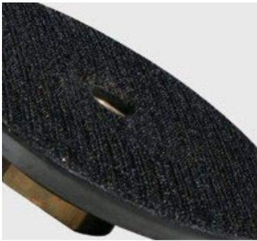
**1. Rigid Backer Pads:** Flexible backers work well for concave profile edges, such as ogee edges. The need to use a flexible backer on most other profiles is not needed. Keep in mind automatic edge machines all use extremely rigid polishing tools and backer pads; these machines will produce a far better edge than what many fabricators can do by hand.
